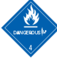
Hazardous Materials Class 4.3: Dangerous when Wet
